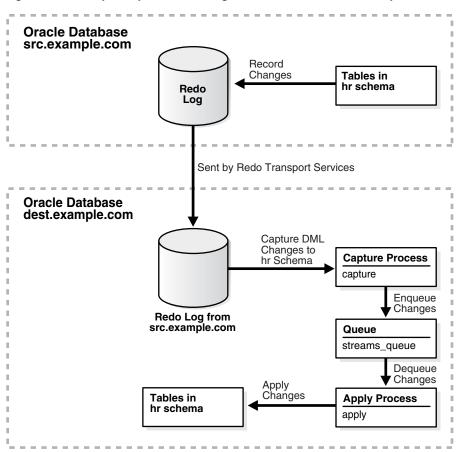
Figure 1–3 Sample Replication Configuration with Downstream Capture
