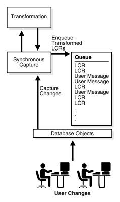
Figure 6–2 Transformation During Capture by a Synchronous Capture
