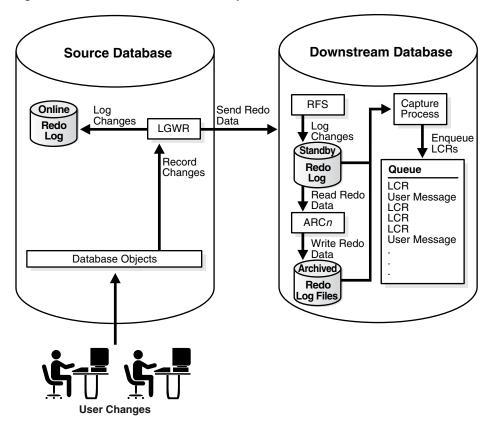
Figure 2–2 Real-Time Downstream Capture
