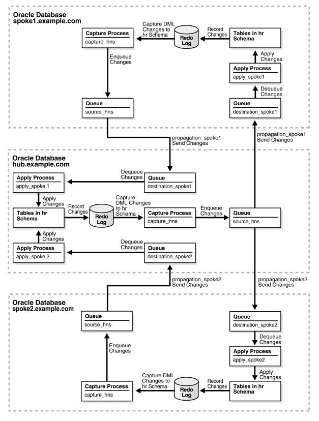
*Figure 1–2 Sample Hub-and-Spoke Replication Configuration*
