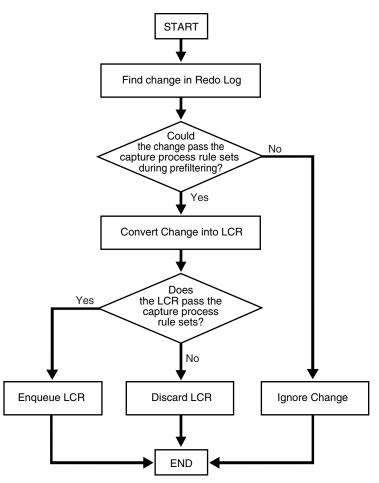
Figure 7–5 Flowchart Showing Capture Process Rule Evaluation
