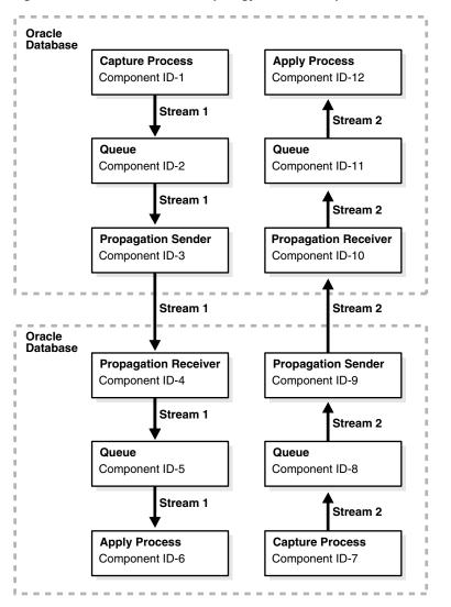
Figure 23–1 Oracle Streams Topology with Two Separate Stream Paths
